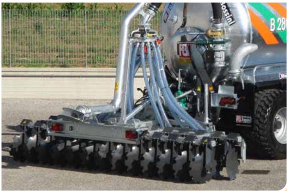
Barra rasoterra applicata al sollevatore per varie dischiere Bar applied to the linkage for various disc equipment
