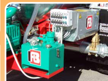
Circuito idraulico indipendente Independent hydraulic system
