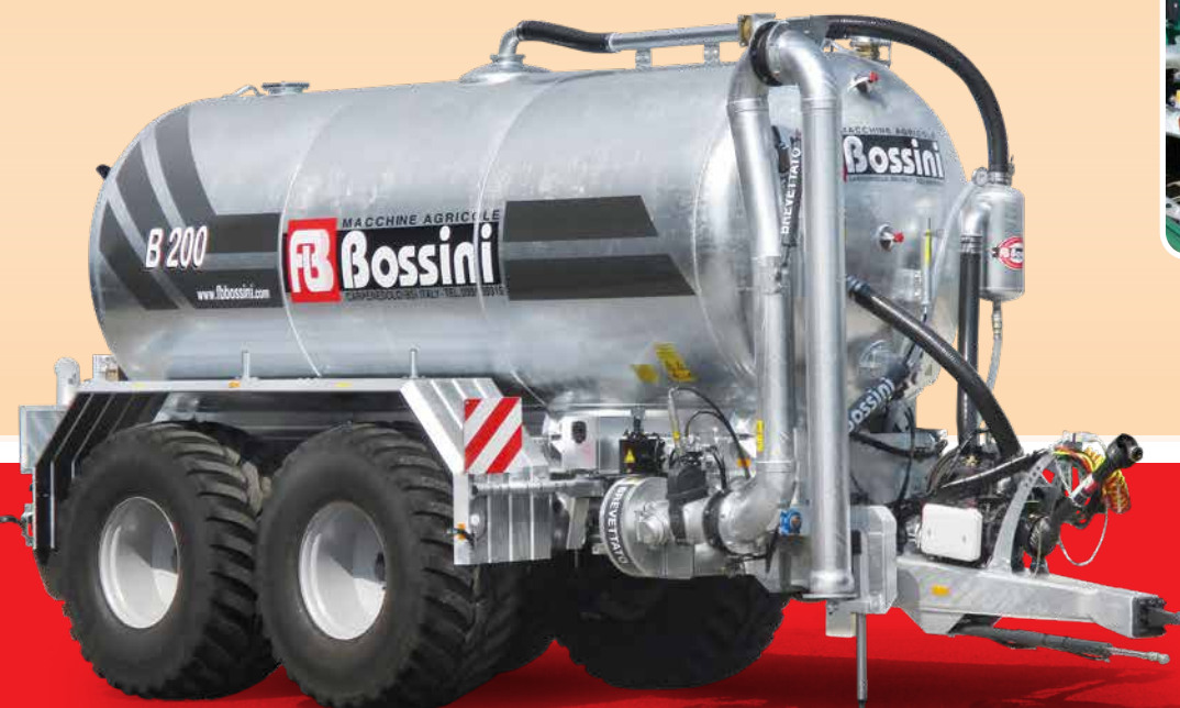
Assale estensibile a comando idraulico mediante n° 2 cilindri a doppio effetto con pattini di scorrimento anti-usura. Extendable axle with hydraulic control by means of 2 double-acting cylinders with wear-resistant sliding pads.
