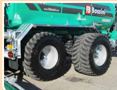
Assale estensibile a comando idraulico mediante n° 2 cilindri a doppio effetto con pattini di scorrimento anti-usura. Extendable axle with hydraulic control by means of 2 double-acting cylinders with wear-resistant sliding pads.
