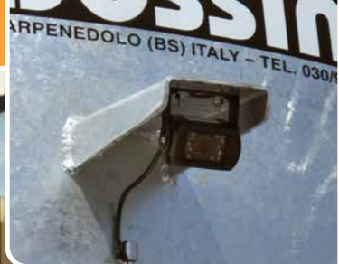
Telecamera ad infrarossi con monitor LCD sulla trattrice Infrared camera with LCD monitor on the tractor
