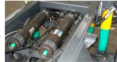
Accumulatori ad azoto a membrana o doppia camera Nitrogen accumulators with membrane or piston-type
