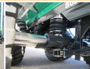
Assale estensibile a comando idraulico mediante n° 2 cilindri a doppio effetto con pattini di scorrimento anti-usura. Extendable axle with hydraulic control by means of 2 double-acting cylinders with wear-resistant sliding pads.
